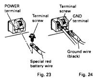
Securely fasten the special red battery lead and the ground wires with terminal
